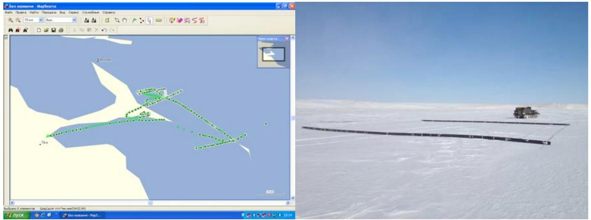
**Figure 5.** Electromagnetic (EM) survey validated by boreholes (penetrated throughout thaw-permafrost sediment) is a new and powerful tool to survey the table of subsea permafrost. Left: tracks of the EM survey -2014; right: the EM system ttawed by the all-terrain vehicle.
