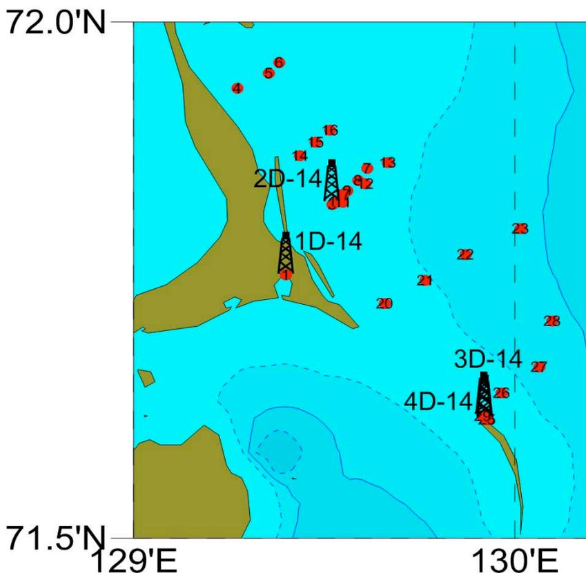
**Figure 1.** Locations of winter drilling/oceanographic/geophysical stations, April 2014: red circles: geophysical (electromagnetic) stations; red-blue circles: complex oceanographic/electromagnetic stations; drilling rigs: drilling sites accompanied by electromagnetic survey.
