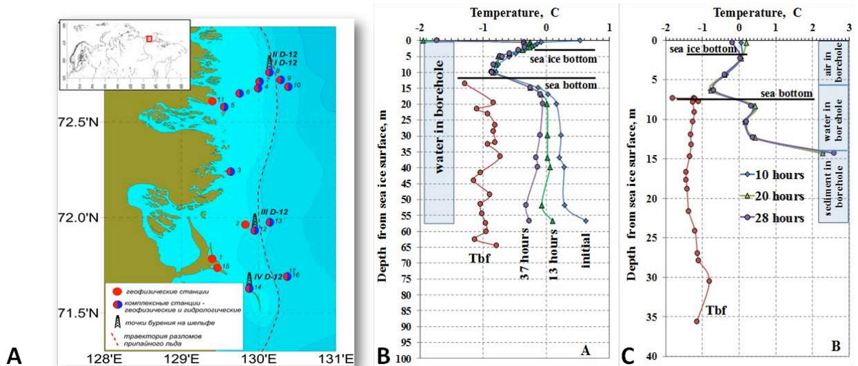
**Figure 3.** A) Position of a borehole drilled in March-April 2012; B) measured temperature along the borehole and estimated freezing temperature in the borehole drilled in April 2011 (marked as 16/17 in A); C) temperature in the borehole drilled in March 2012 (marked as 2D-12 in A); “Tbf” means “temperature at beginning of freezing” (Semiletov et al., 2014, in preparation).
