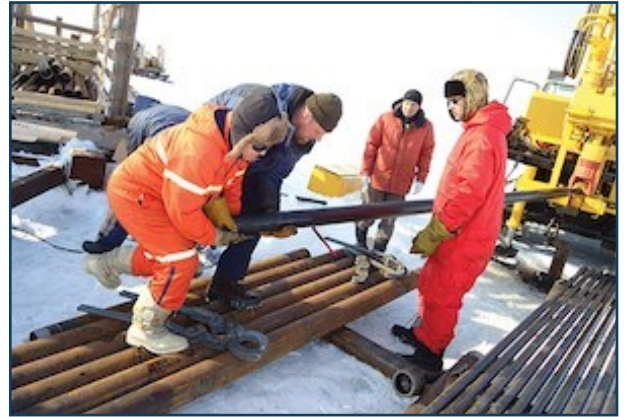
Members of the East Siberian Arctic Shelf scientific research expedition drill into sub-sea permafrost under fastice. Photo by Igor Semiletov.
