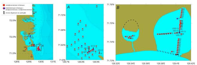
*Figure 2*. Locations of winter drilling/oceanographic/geophysical stations, April 2013: red circles: geophysical (electromagnetic) stations; red-blue circles: complex oceanographic/electromagnetic stations; drilling rigs: drilling sites accompanied by electromagnetic survey.
