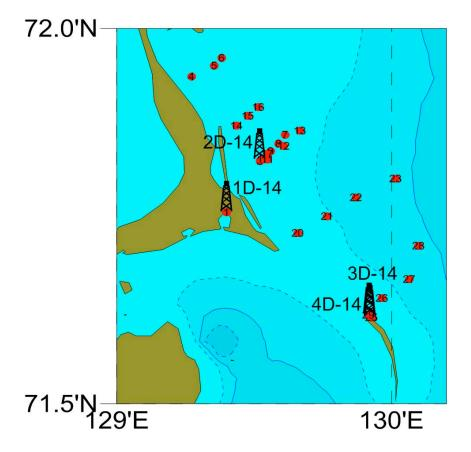
**Figure1**. Locations of winter drilling/oceanographic/geophysical stations, April 2014: red circles: geophysical (electromagnetic) stations; red-blue circles: complex oceanographic/electromagnetic stations; drilling rigs: drilling sites accompanied by electromagnetic survey.
