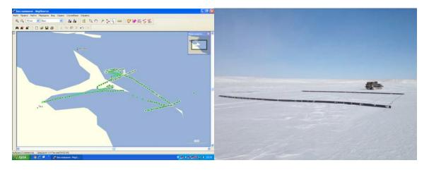
**Figure 5.** Electromagnetic (EM) survey validated by boreholes (penetrrated throughout thawpermafrost sediment) is a new and powerful tool to survey the table of subsea permafrost. Left: tracks of the EM survey -2014; right: the EM system ttawed by the all-terrain vehicle.
