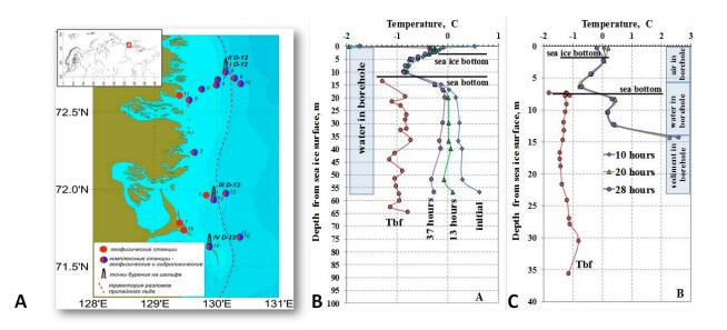
**Figure 3.** *A)* Position of a borehole drilled in March-April 2012; B) measured temperature along the borehole and estimated freezing temperature in the borehole drilled in April 2011 (marked as 16/17 in A)); C) temperature in the borehole drilled in March 2012 (marked as 2D-12 in A)); "Tbf" means "temperature at beginning of freezing" (Semiletov et al., 2014, in preparation).
